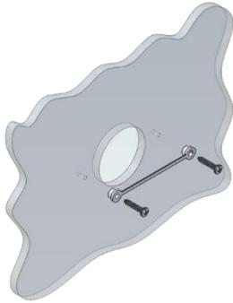
**Step 1:** Locate the mounting buttons horizontally across the hole with the smaller diameter against the wall.
