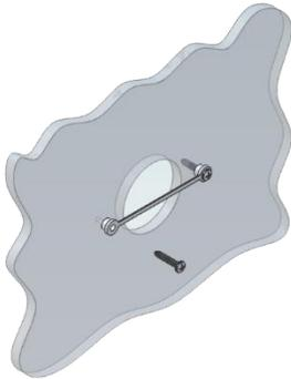
**Step 2:** Screw in one screw and level the buttons so the display will be straight when installed.
