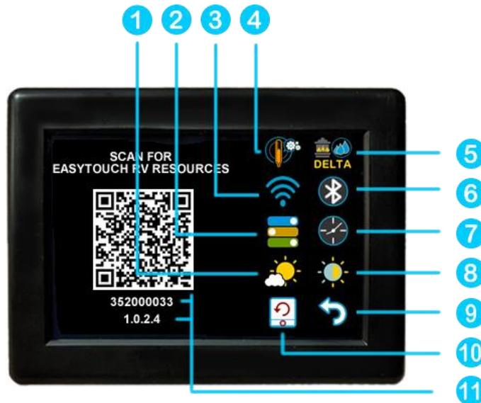
1. Day/Night mode. Day mode (shown above) will dim the display down to the screen saver set point after 30 seconds. Night mode (moon icon) will turn off the back light after 30 seconds. The display will brighten again once the touch screen is pressed. See (7) to set brightness.
