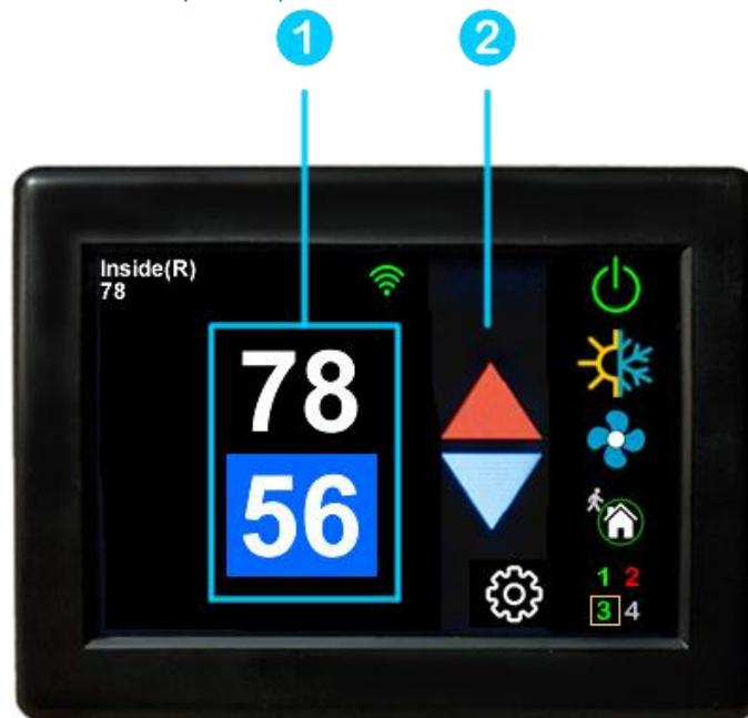
Away operation allows setting upper and lower limits for temperature with a non-operating area or “dead band” in the middle. This can be useful when setting a higher daytime cooling temperature and lower night time heating temperature. It can also be used to control the temperature extremes when you are away from the RV. The mode selected must be an automatic mode to allow both heating and cooling operation.
