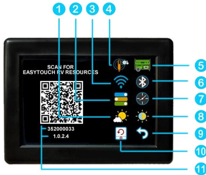
1. Day/Night mode. Day mode (shown above) will dim the display down to the screen saver set point after 30 seconds. Night mode (moon icon) will turn off the back light after 30 seconds. The display will brighten again once the touch screen is pressed. See (7) to set brightness.
