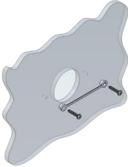
**Step 1:** Level the mounting bracket horizontally across the hole with the smaller diameter of the mounting button against the wall.
