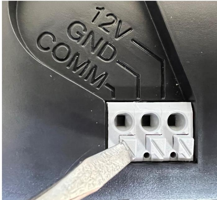
*Figure 3 - EasyTouch RV Wire Terminals*
