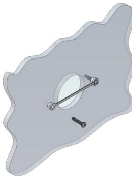
**Step 2:** Screw in one screw and level the buttons so the display will be straight when installed. Screw into the smaller hole of the two buttons.
