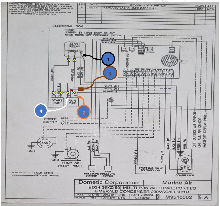
NOTES: First remove the orange & white wires (yellow x's) from the start relay/start cap
