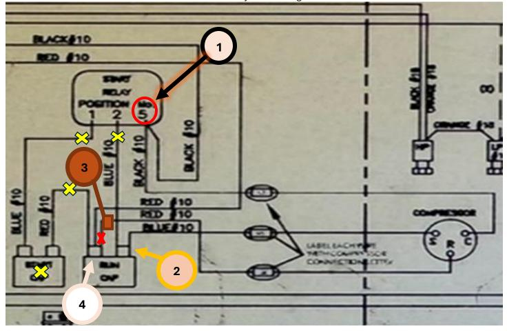
NOTES: Disconnect the wires and components with the yellow x's. The DDC circuit board is not touched during Easy Start installation.
