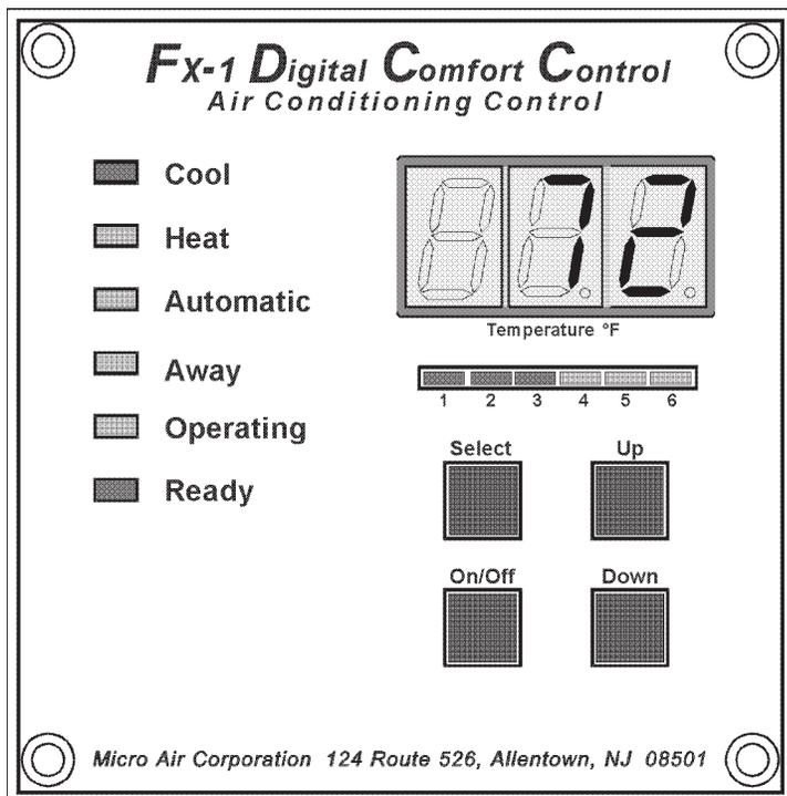
**UP BUTTON** Momentarily press and the set point will appear in the temperature display. The set point increases one degree each time the up button is pressed and released.
