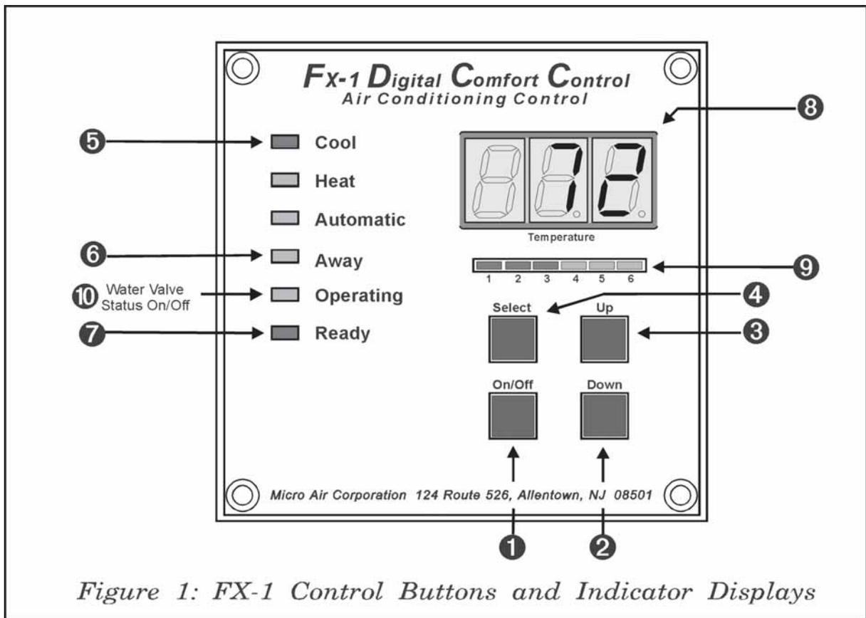
Figure 1: FX-1 Control Buttons and Indicator Displays
