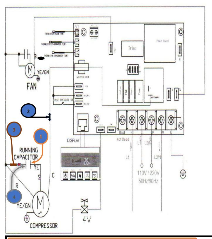
1) Attach the Easy Start Orange wire here with the existing compressor start (S) wire
