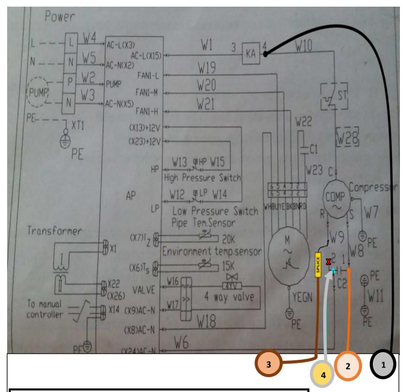
1-Make a 3-way splice with the Easy Start Black wire & anywhere along the W10 comp C wire
