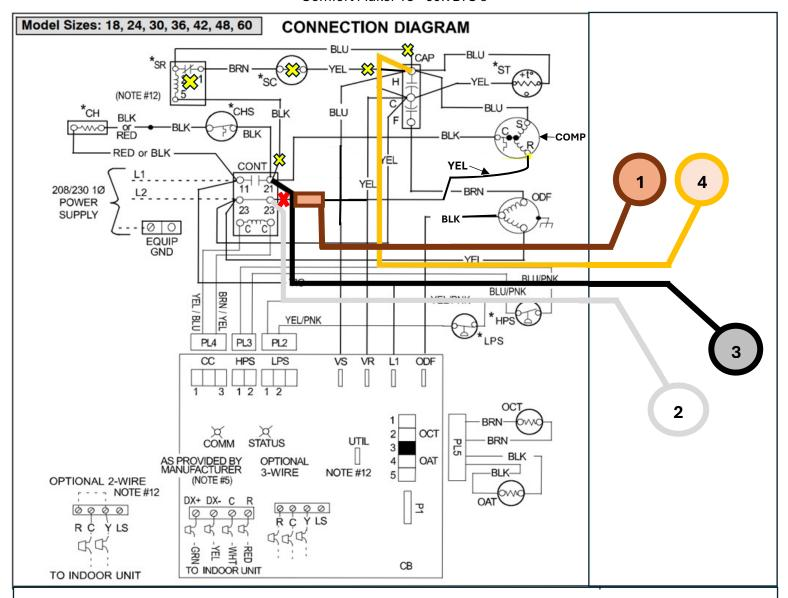
NOTES: Any optional components installed, marked with yellow x's, need to be removed before ES installation
