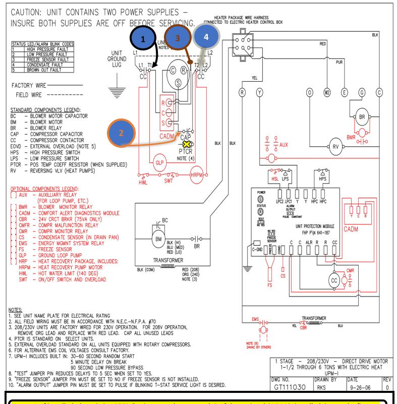
Notes: A. If installed, the existing PTCR & wires must be removed. B. If the optional CADM is installed, it must be first set up according to the directions in the Residential Installation Manual on page 4
